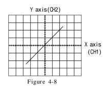
Note: When high frequency signals are displayed in the X-Y operation, pay attention to the frequency bandwidths and phase difference between X and Y-axis.
